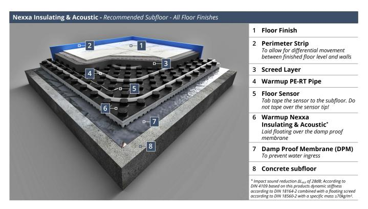
Warmup Nexxa Insulating & Acoustic panels are intended for multi-residential dwellings. Its thermal insulation performance is sufficient to meet the requirements of separating floors defined within EN 1264 and ISO 11855
